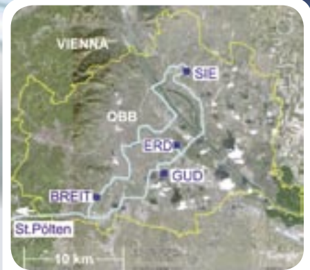
City map of Vienna and the SECOQC network. The optical fiber ring connects the nodes, which host the network node modules and the QKD devices.
